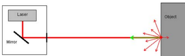
Fig. 1 Measuring principle of a terrestrial laser scanner. Left: The mirror inside the laser scanner that deflects the laser signal in a certain direction. Right: The measured object on which the signal is reflected. The green arrow is the echo returning to the laser scanner
